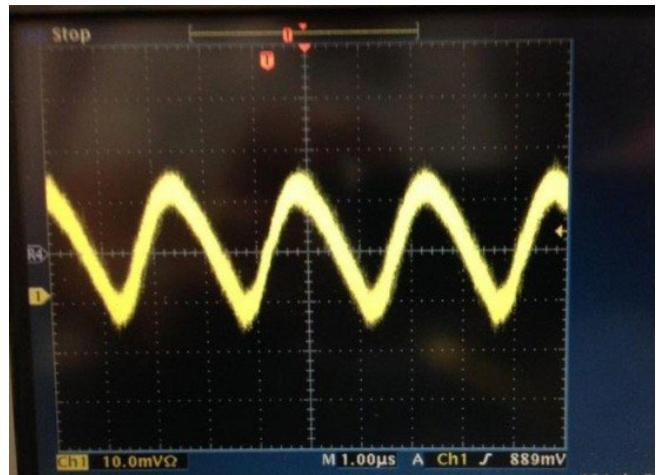
Measuring the same signal on another brand of oscilloscope shows so much noise that the details of the signal become lost, negatively impacting the credibility of the data
