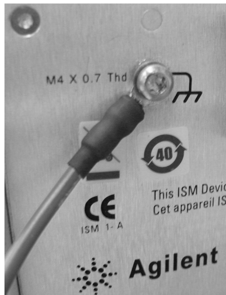
Figure 3-17 EMC grounding cable attached to VXI main frame chassis
