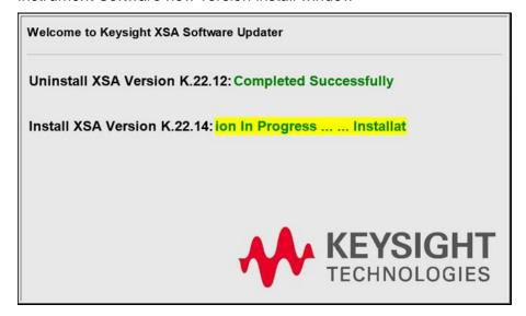
The new instrument software is being installed. The installation in progress will roll across the screen indicating software activity. There may be several windows appearing and disappearing during this time. Updating the installed boards FPGA code. This will take a long time to update each installed board. NO interaction with the Wideband Transceiver is required.
