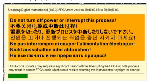
**NOTE:** The instrument is configured to have at least 2 LO boards installed. Updating the FPGA code on each board can take about 10 Minutes.
