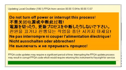
This Screen will appear and disappear for each LO board installed. It may appear as a Loop but, it is dependent on the number of LO boards installed. Please be patient. The green progress bar will roll across the screen indicating software activity.
