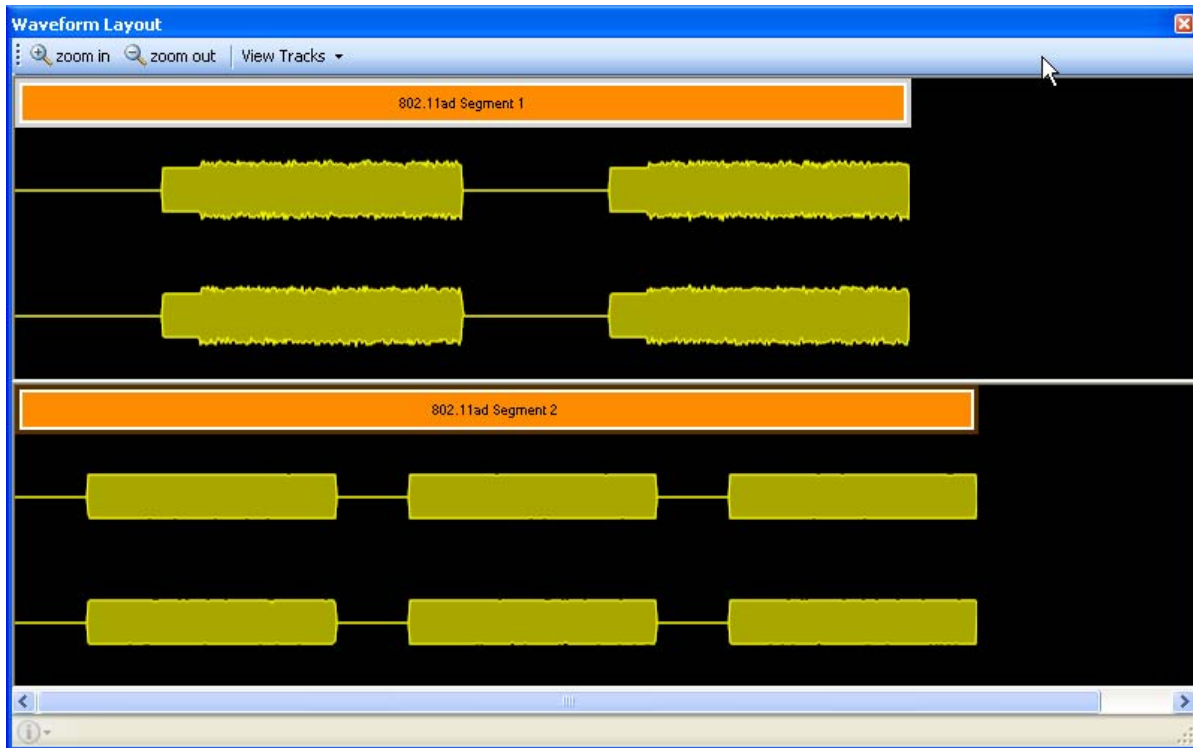
Figure 31. Waveform Layout for Modulated Interferer
