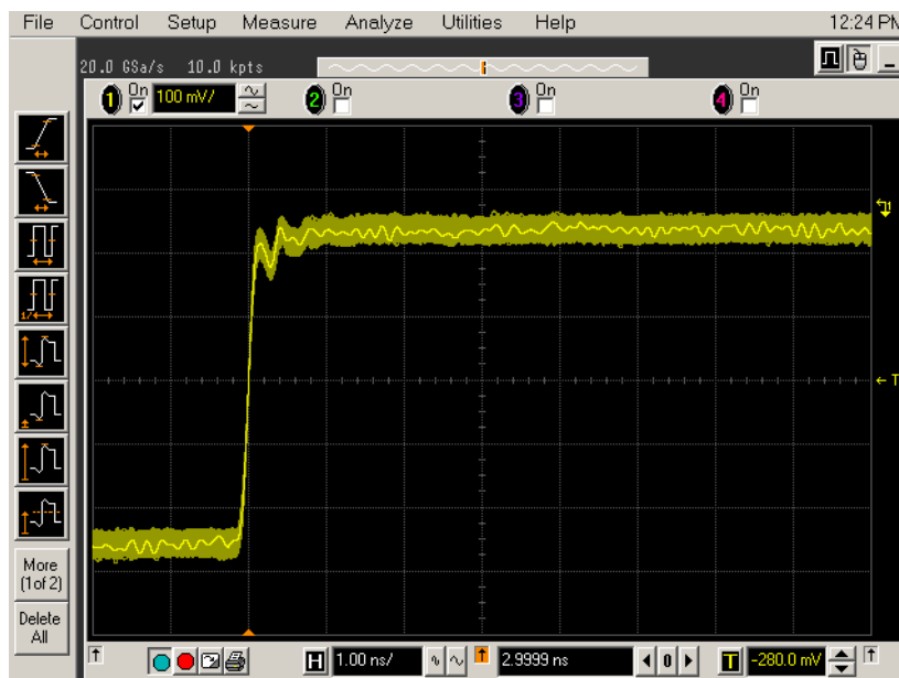
Figure 25 Good Connection Waveform Example
