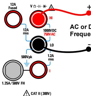
AC or DC Voltage Capacitance, Continuity Diode Test Frequency, Resistance, or Temperature Measurements
