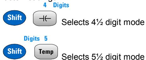
Note: The continuity and diode test functions have a fixed, 4½ digit display. Capacitance and temperature have a fixed, 3½ digit display.
