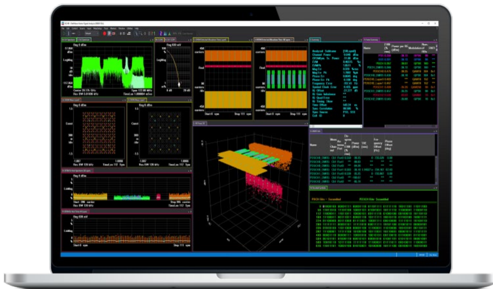
Figure 1. Keysight RF capture and analysis software supports automated verification in scalable EWASP test environments.
