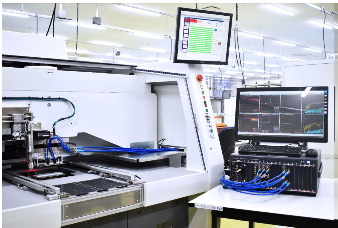
Figure 1. Yamaha micro prober system with the M980xA PXI VNA
