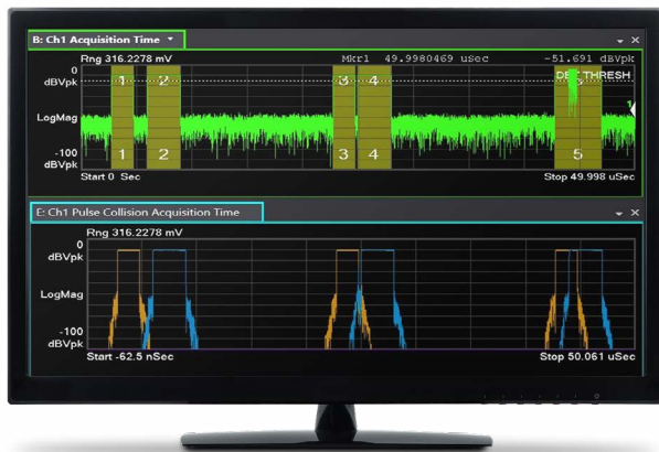
Figure 11. Pulse collision analysis enables users to differentiate between friendly, neutral, and hostile emitters, even when their signals overlap.
