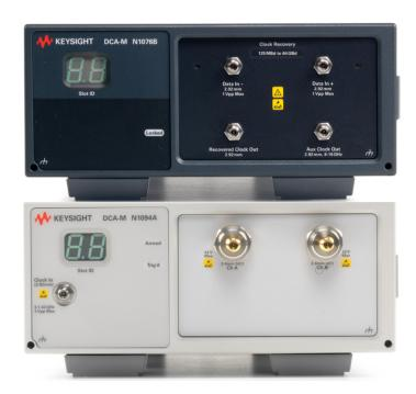
The N108xA software also supports a variety of other DCA configurations (see ordering guide), including the N1094A DCA-M oscilloscope and N1076B Electrical Clock Recovery.
