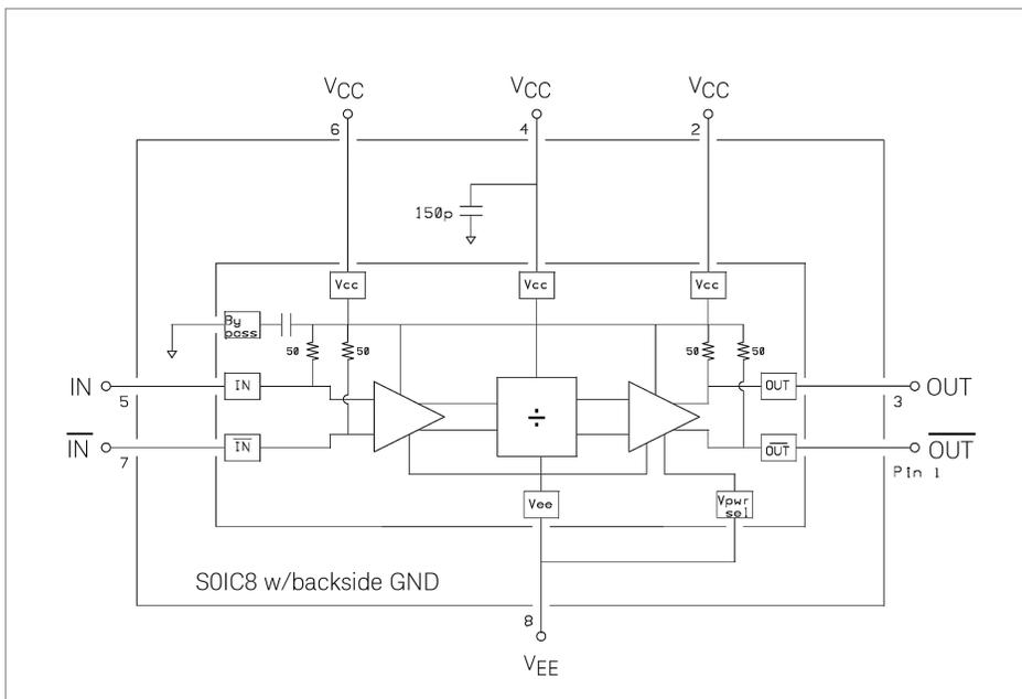
Figure 1. Simplified schematic diagram
