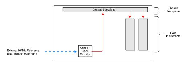
All chassis have on their rear panel a 10MHz reference BNC input and a 10MHz reference BNC output. In the case of the M904x chassis, there are two Reference clock SMA outputs on the front panel.
