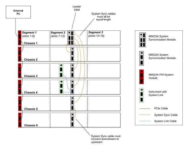
This following code shows how to use the HVI Python API to define and use the SSMs in the multichassis system shown in the diagram. Each System Sync Downstream port connects to the System Sync Upstream port of another System Sync Module in a different chassis.
