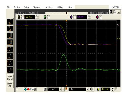
The following picture shows the desired effect of no skew between the cables. Note that the channel 1 (yellow trace), channel 3 (purple trace) traces overlap, and the differential signal (green trace) is flat. If this is not the case, then perform the following steps to reduce the skew between channels 1 and 3.
