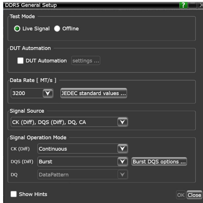
Figure 6 DDR5 General Setup window
