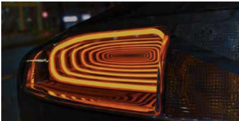
Figure 8. Lit appearance image created in the LucidShape Visualize Module
