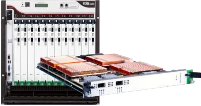
Figure 1. Data Center Storage 100GE Test Load Module with 2x100GE QSFP28 Ports
