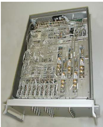
Figure 2. RF signal conditioning and switching
