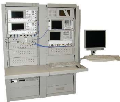
Figure 3. RF Test System with Multiple Custom Switch Matrices
