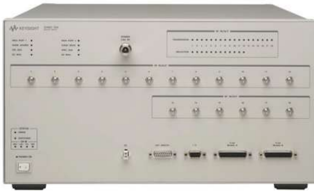
Figure 8. Fully assembled custom switch matrix
