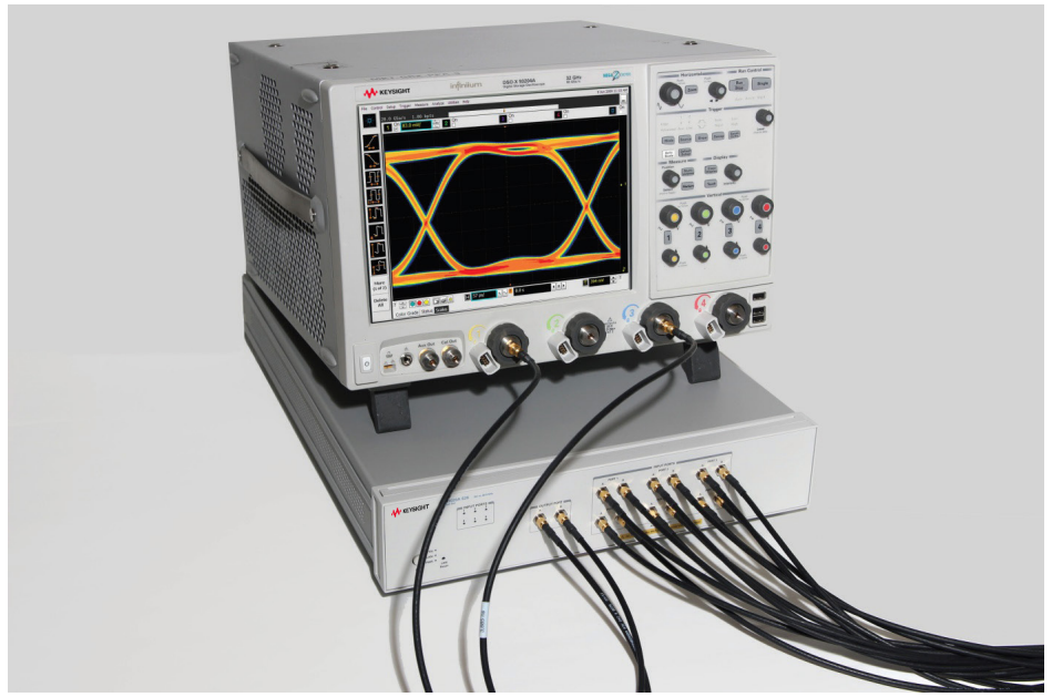
Figure 13. Automated testing for multi-lane digital bus interface through switching solution.
