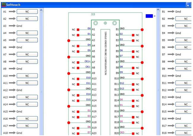
To map a signal bit to a pin, click the signal box displayed in front of that pin in one of the two columns on left or right of the diagrammatic representation.
