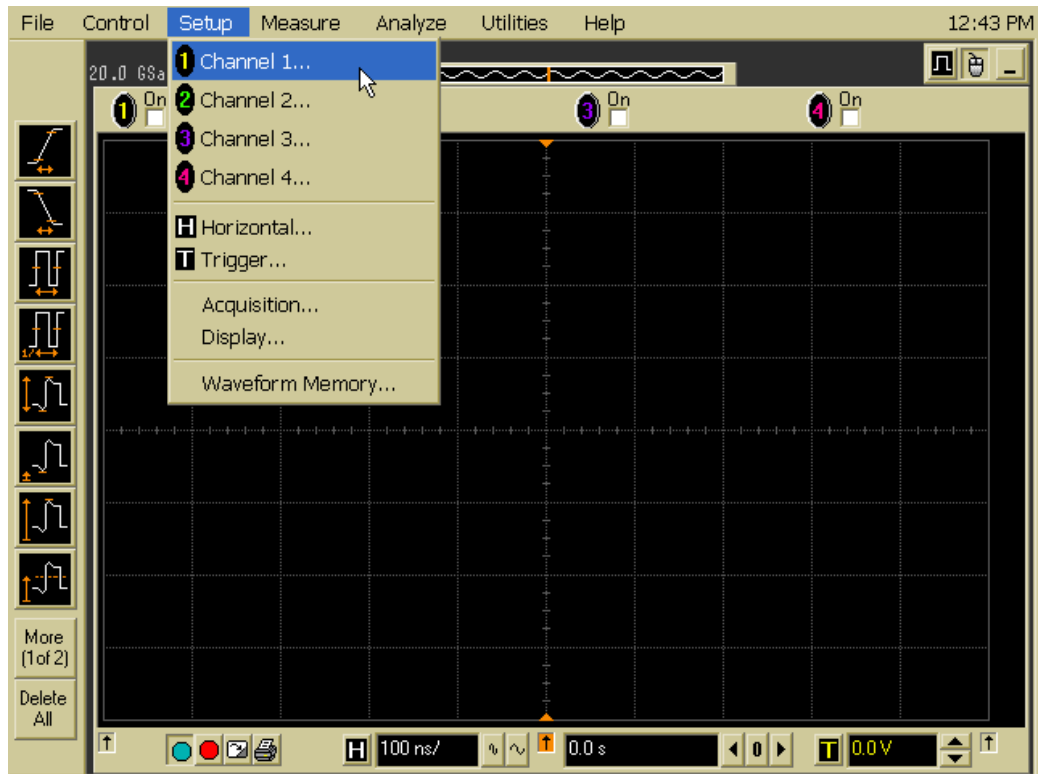
Figure 20 Channel Setup Window.
