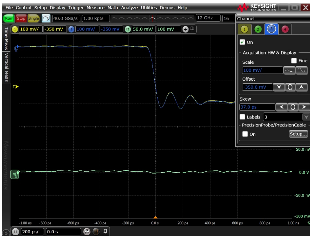
Figure 40 No Channel-to-Channel Deskew
