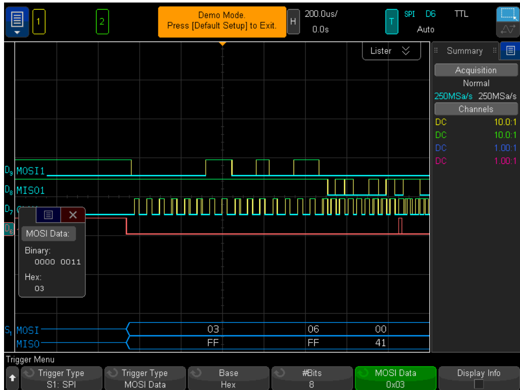
Figure 57 Triggering on MOSI data = 03 HEX .
