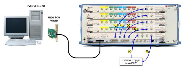
Figure 4 System level cabling of a sixteen channel synchronous system
