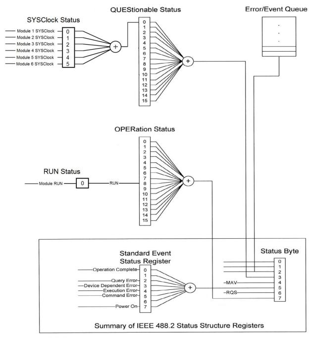
Figure 15 Status Register Structure
