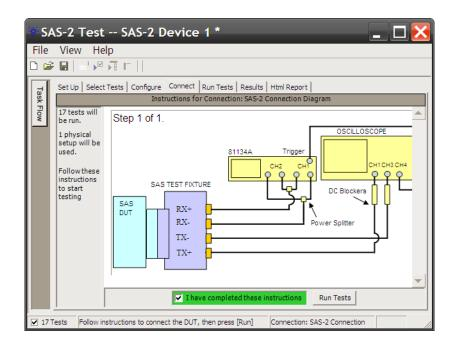
3 When connections to the device under test have been made, check the I have completed these instructions box.
