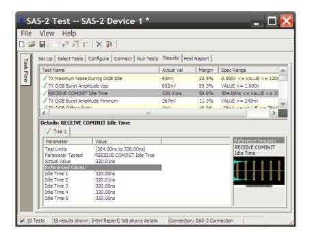
The Results tab contains three resizable panes for test results information. If you select one of the tests in the top pane, details and reference images (if any) are shown in the lower panes.
