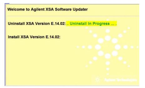
The old instrument software is being removed. The "Uninstall in Progress" text will roll across the screen indicating software activity. There will be several windows appearing and disappearing. It will display "Completed Successfully" when this step is finished.
