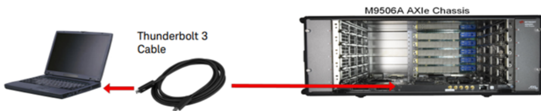
Figure 3 Connecting an External Laptop PC to the M9506A with Thunderbolt 3
