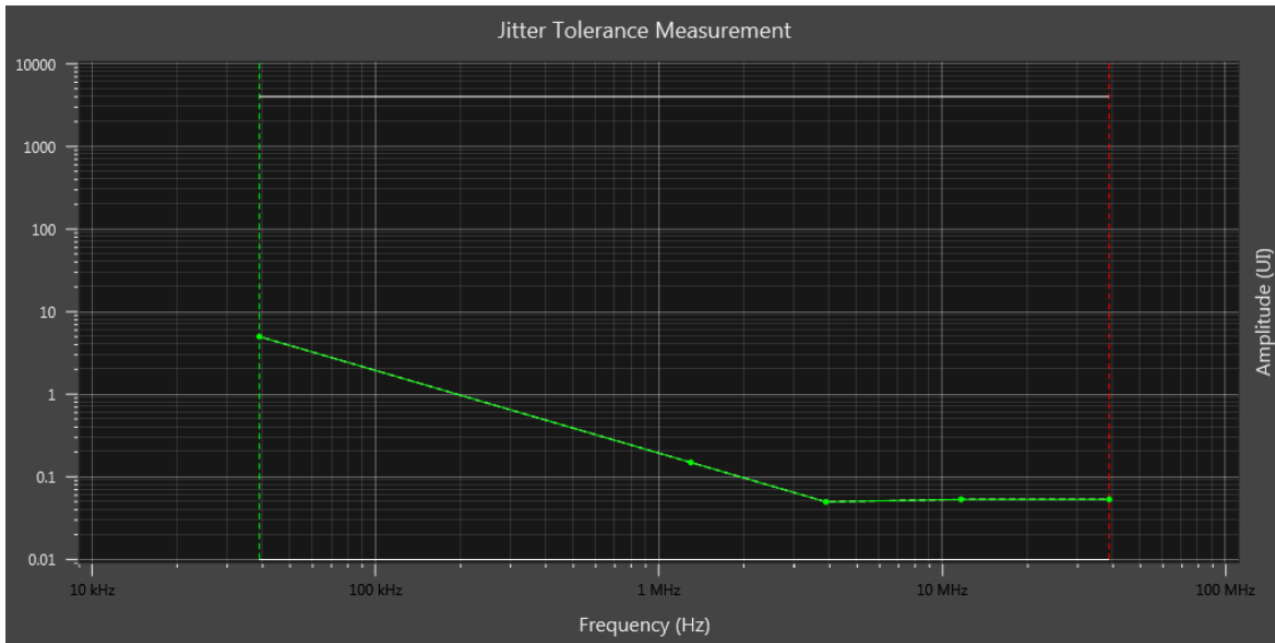
Figure 53 VSR Host Single-lane Stressed Input Test Result (graphical)
