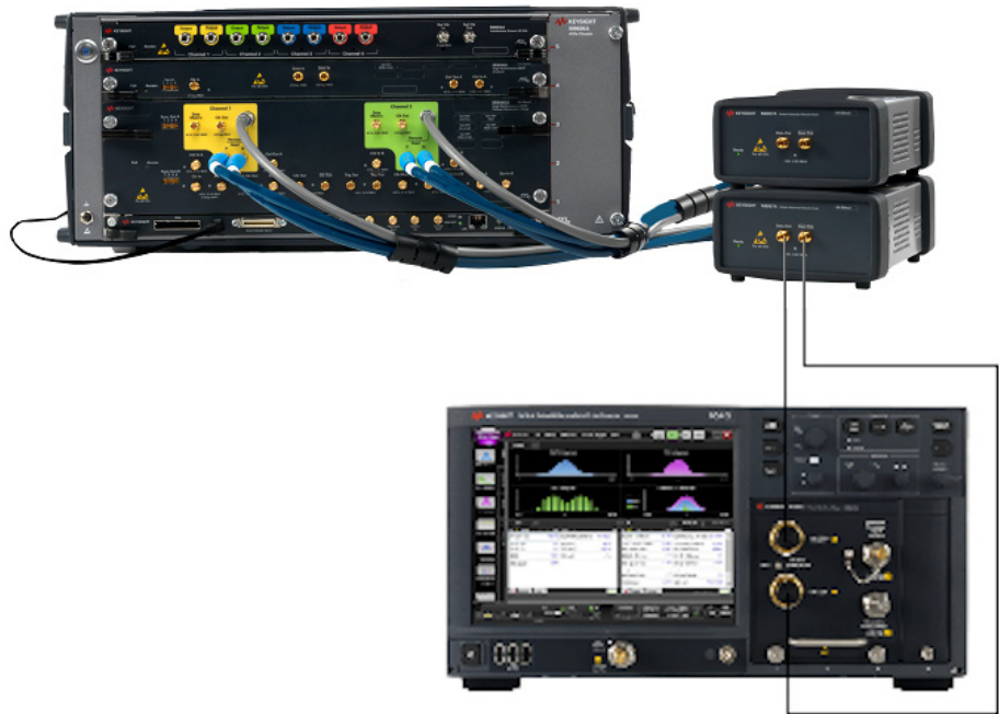
Figure 71 Amplitude Calibration connections for MR
