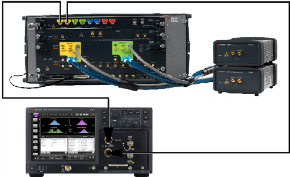
Figure 80 Broadband Noise Calibration connections for MR
