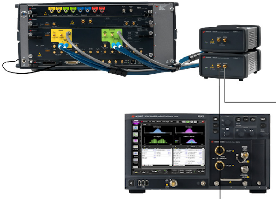
Figure 97 SJ Calibration connections for LR
