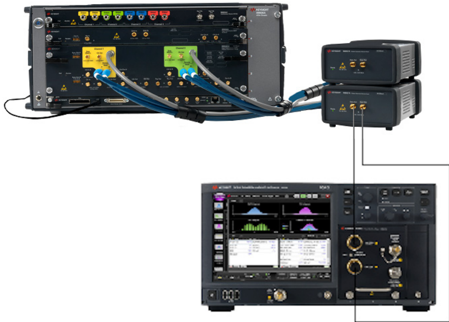
Figure 37 UUGJ Calibration connections for VSR Host & VSR Module
