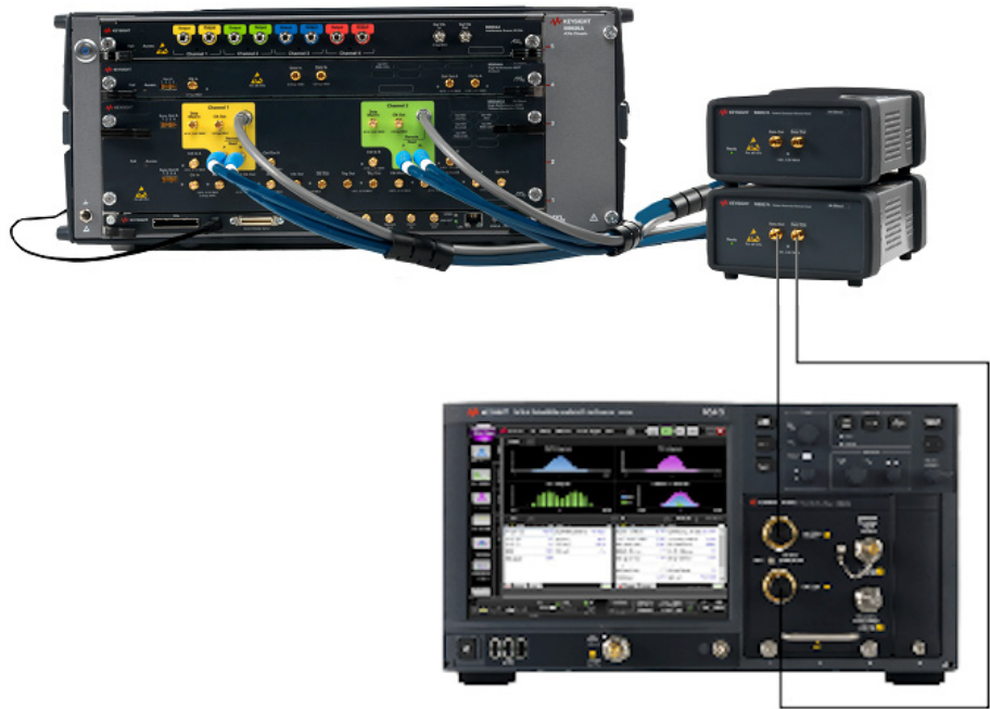
Figure 94 Amplitude Calibration connections for LR
