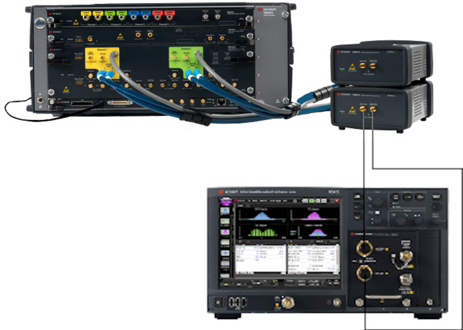
Figure 82 Transmitter Measurements for COM Model connections for MR
