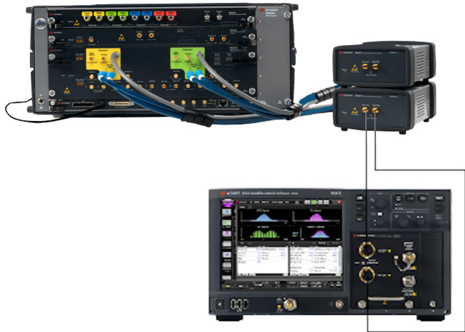
Figure 84 Transmitter Measurements for COM Model connections for MR
