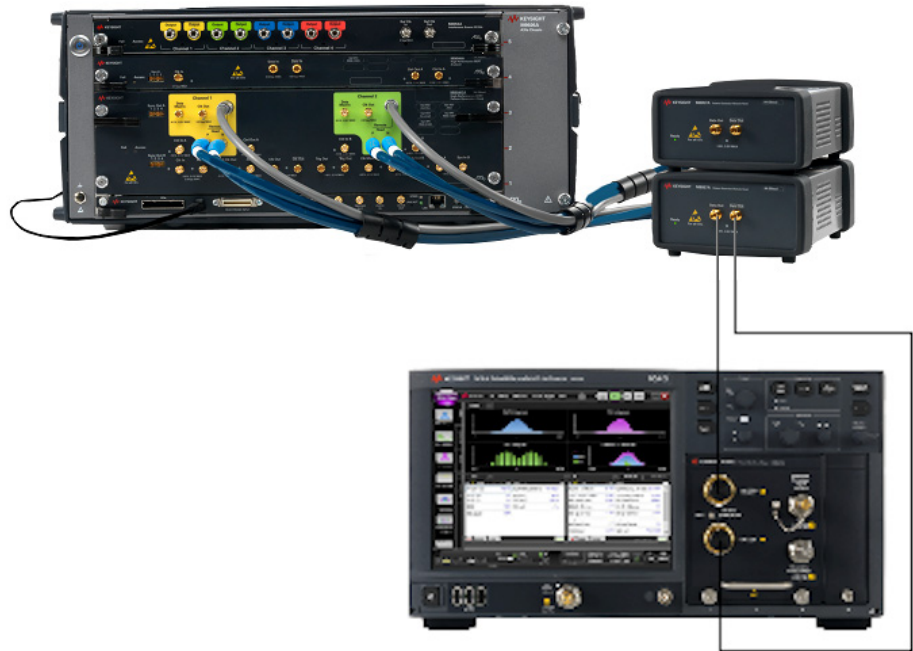
Figure 109 Transmitter Measurements for COM Model connections for LR
