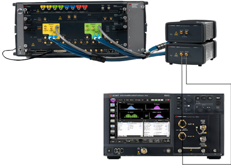
Figure 77 UUGJ Calibration connections for MR
