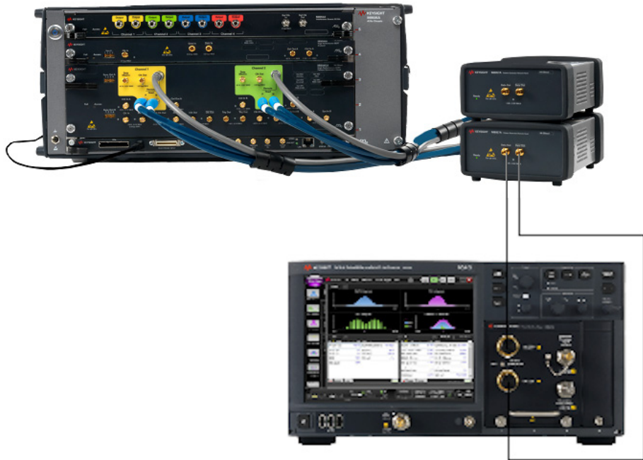
Figure 100 UUGJ Calibration connections for LR
