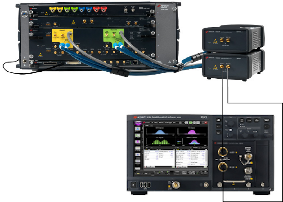
Figure 116 Transmitter Measurements for COM Model connections for LR
