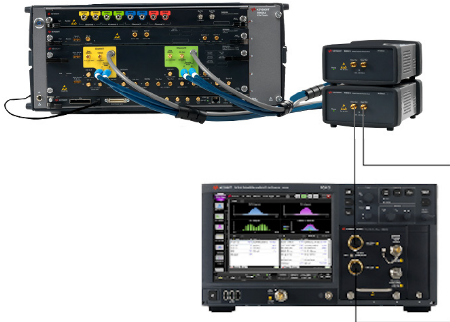
Figure 74 SJ Calibration connections for MR
