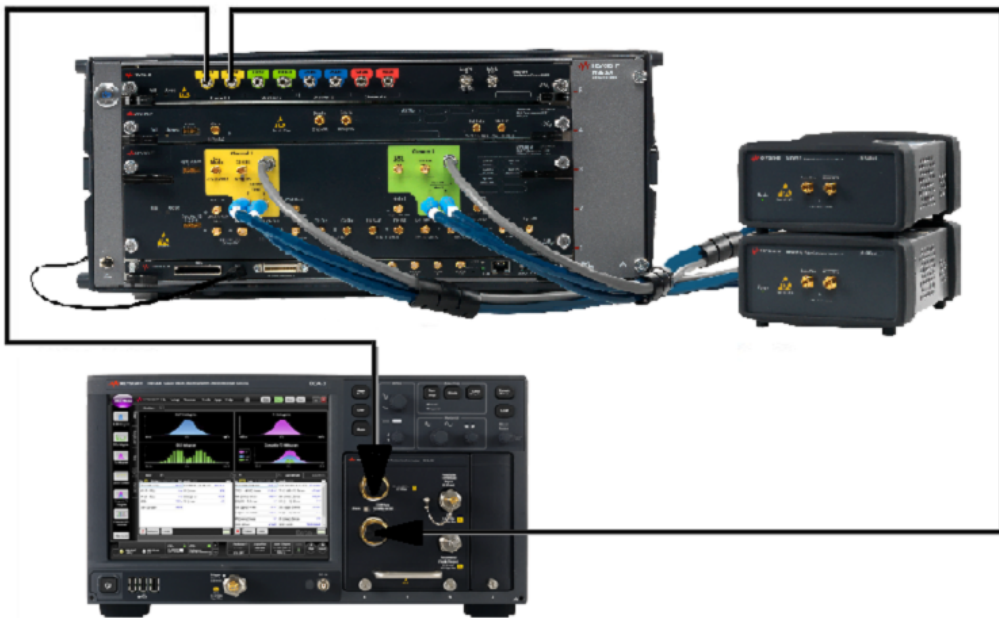
Figure 103 Broadband Noise Calibration connections for LR
