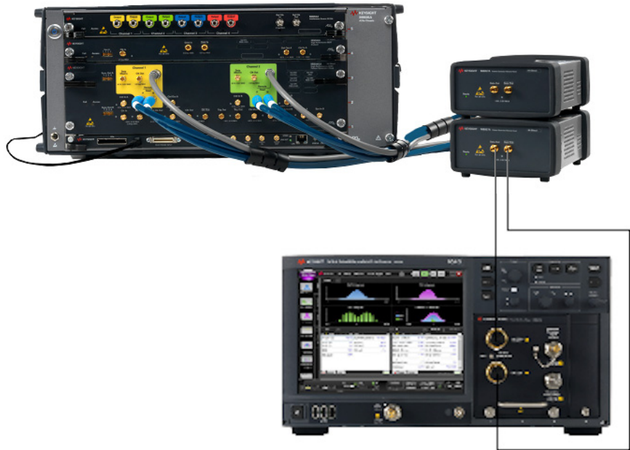
Figure 34 SJ Calibration connections for VSR Host & VSR Module
