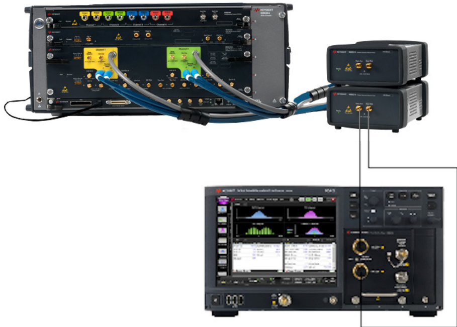
Figure 31 Amplitude Calibration connections for VSR Host & VSR Module
