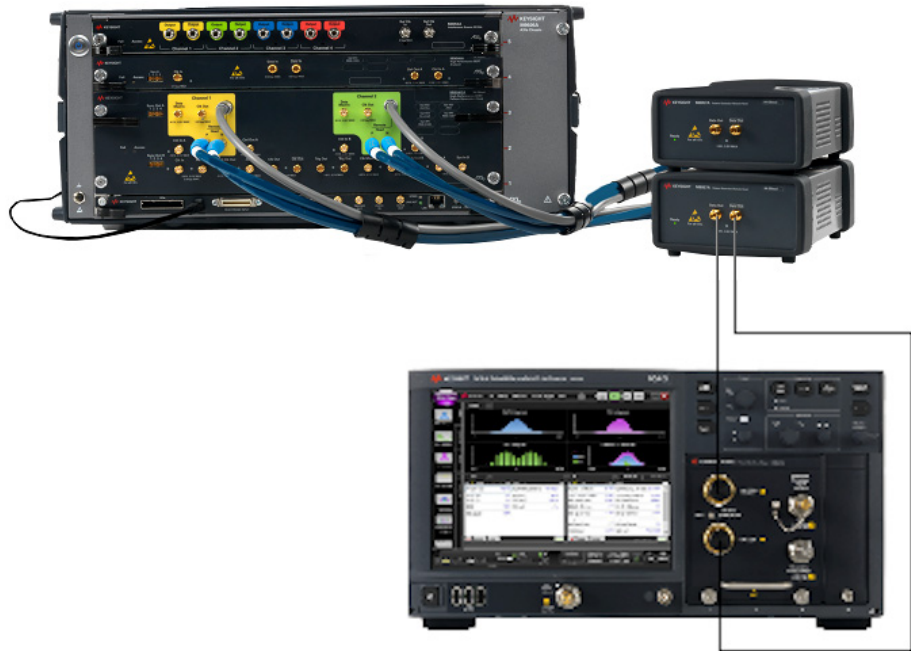
Figure 40 BUJ Calibration connections for VSR Host & VSR Module
