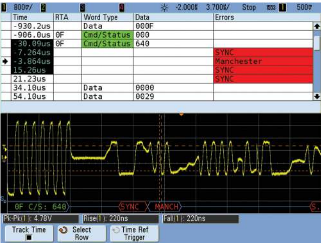
Figure 5. MIL-STD 1553 error triggering helps to uncover signal integrity problems.
