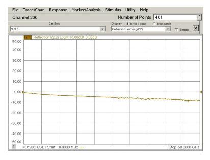
Figure 48 Typical Reflection Tracking Trace (Ports 5 to 8)
