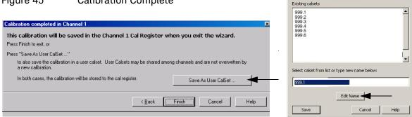
**6.** Repeat steps 1 thru 5 for Ports 2 thru 16. When finished, there should be 16 Cal Sets saved with the titles "999.1" thru "999.12" (12-Port).
