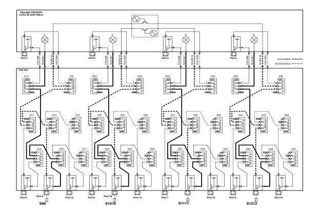
Figure 18 Typical Reflection Response Ports 13 to 16
