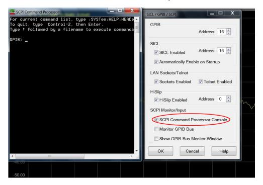
Figure 37 Command Console for 'B' Model Analyzers
