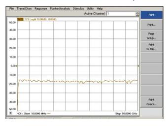
Connect the RF Flex cables to the Source IN and CPLR THRU Port Connect the RF Flex cables to the Source IN and CPLR THRU port indicated in Table 20, the expected results should be similar to Figure 62.
