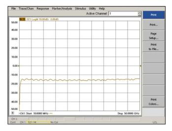
Figure 60 RCVR OUT to Ports 9-12 Path Response
