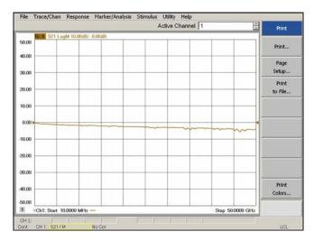
Figure 57 Source IN to Ports 9-12 Path Response
