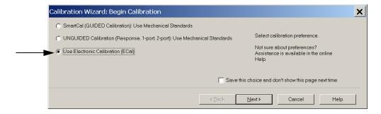
2. Continue following the Cal Wizard prompts. In the Select Calibration Ports and ECal Module dialog box click the Select All, check box, or select the ports you are calibrating and click Next. If an ECal characterization has been done, select View/Select ECal Module and select the previously saved user file from Step 1.
