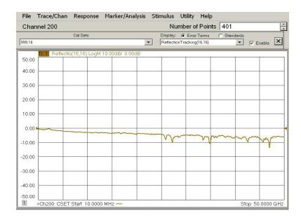
If you are using an ECal module you can verify the individual port calibration.
