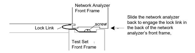
8. Secure the analyzer's lower lock-links to the test set's upper lock-link using the spring-loaded screws. If the analyzer's lock-links are not aligned with the screw holes, loosen the screws securing the feet to the instrument slightly to align and tighten.
