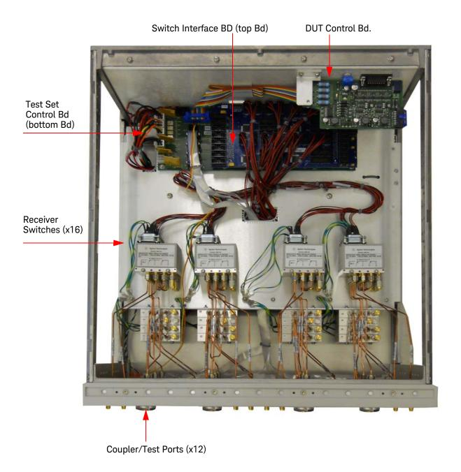
Figure 64 Test Set Bottom View
