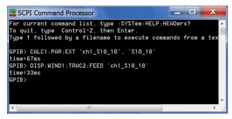
This first command creates a new S10\_10 measurement on channel 1 of the PNA-X, named "ch1\_S10\_10," and configures the internal Test Set RF switches.
