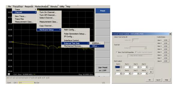
This menu will allow the physical Ports 1 thru 16 to be identified as any port for your convenience. Select the Port Control down arrow for Ports 9 thru 16. For example, Port 5 can be re-named Port 2.
