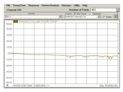
Figure 50 Typical Reflection Tracking Trace (Ports 13 to 16)
