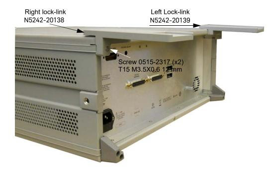
7. Place the analyzer on top of the test set and ensure that the front frame of the analyzer is positioned slightly forward of the locks that are attached to the test set. Slide the analyzer back so the locks engage the front frame of the analyzer.
