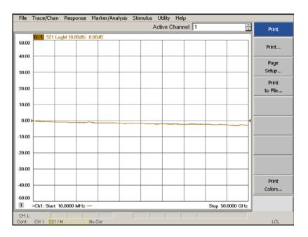
Connect the RF Flex cables to the RCVR OUT and CPLR ARM Port Connect the RF Flex cables to the RCVR OUT and CPLR ARM port indicated in Table 21, the expected results should be similar to Figure 62 on page 80.
