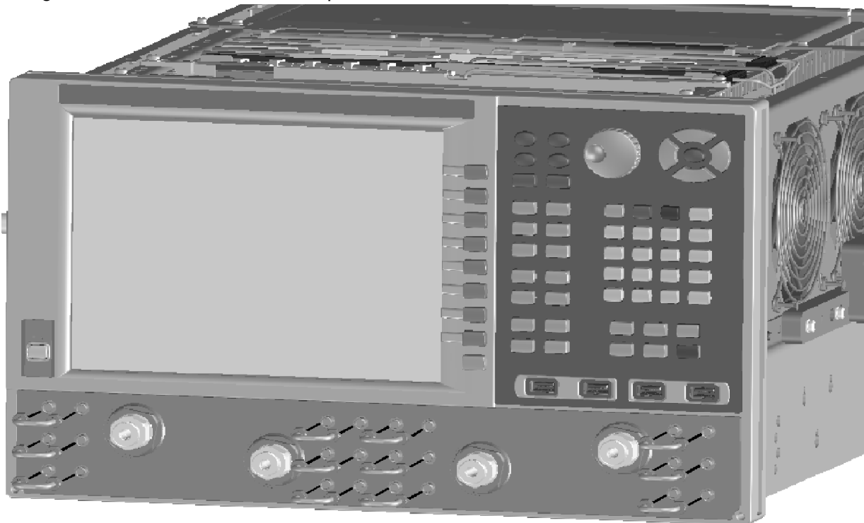
Figure 6 Front Panel Jumper Cables Installation
