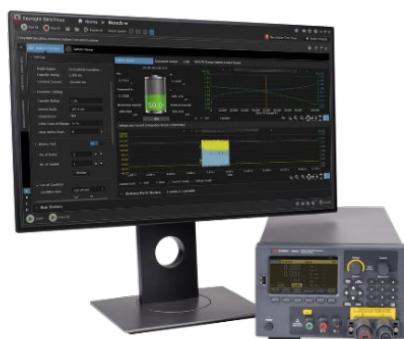
E36731A Battery Emulator with Native Two-Quadrant Operation and BV9211B Software Support
