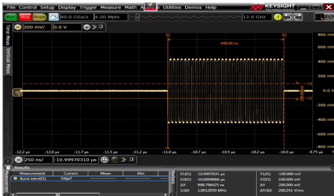
Figure 12 Burst Width Measurement
