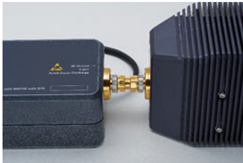
Figure 4 LCA Optical Receiver and Test Set Controller connected to a Network Analyzer
