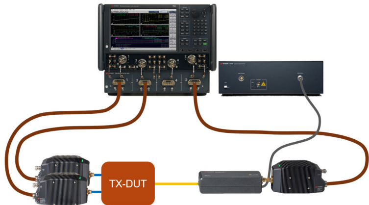
Figure 28 Differential EO measurement setup
