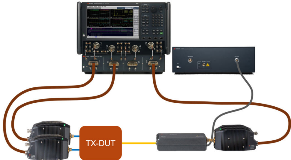
Figure 12 Schematic measurement setup for differential EO measurements
