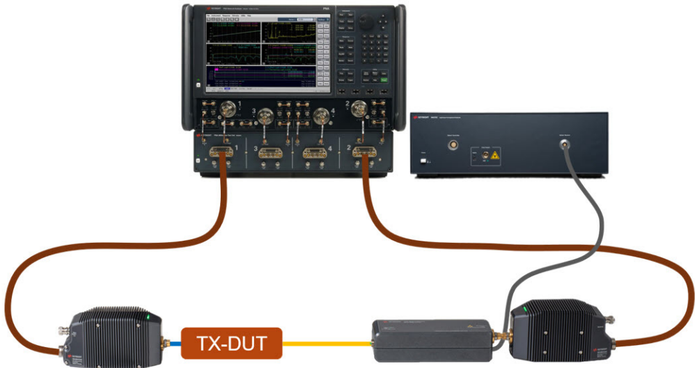
Figure 10 Schematic measurement setup for single-ended EO measurements
