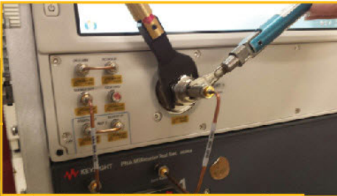
Figure 3-10 N5290/1A-202–(Interconnect Kit N5292-60013): Install semirigid cables (N5292-20014 and N5292-20017) and if not done, connect 50 ohm loads (0955-2394) to the front panel of the PNA and N5292A
