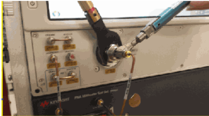
Figure 3-7 To avoid damaging your RF ports 1/2/3/4, always use two wrenches
