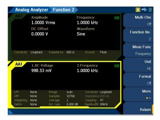
Figure 4-9 Analog Analyzer > Functions > Frequency menu page 1
