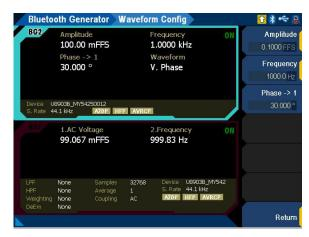
**Figure 3-9** Bluetooth Generator > Waveform Config menu page (variable phase waveform)
