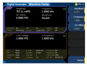
Figure 3-33 Digital Generator > Waveform Config menu page (square waveform)
