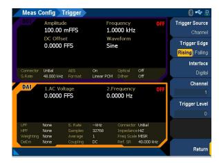
Figure 4-60 Digital Analyzer > Meas Config > Trigger menu page
