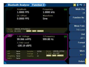
Figure 4-32 Bluetooth Analyzer > Functions > THD level menu page 1
