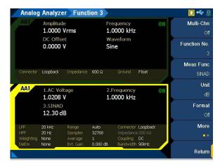
Figure 4-24 Analog Analyzer > Functions > SINAD menu page 1
