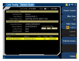
Figure 3-62 Bluetooth Analyzer > Link Config > Device Scan menu page
