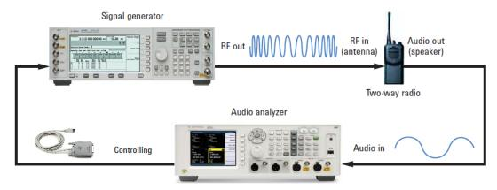
Figure 7-53 General setup for the receiver sensitivity measurement
