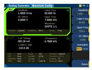
Figure 3-13 Analog Generator > Waveform Config menu page (SMPTE 1:1 waveform)
