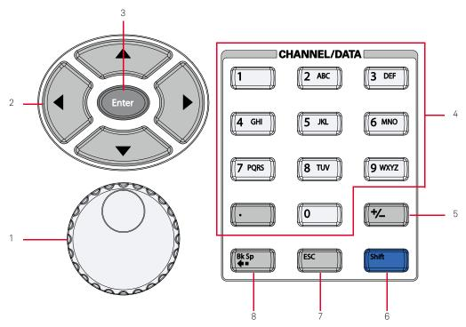
Figure 2-7 Navigation and CHANNEL/DATA panels
