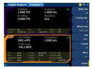
Figure 4-31 Digital Analyzer > Functions > THD level menu page 1
