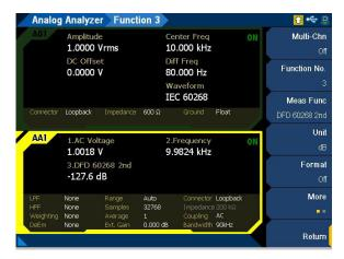
Figure 4-36 Analog Analyzer > Functions > DFD 60268 2nd menu page 1
