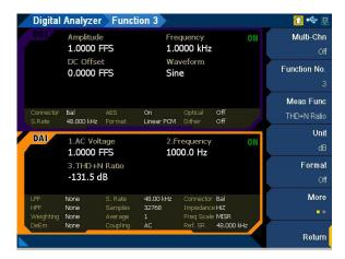
Figure 4-19 Digital Analyzer > Functions > THD+N Ratio menu page 1
