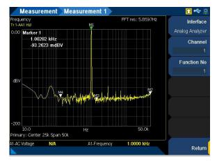
Figure 5-16 Graph Analysis > Measurement > Measurement 1 menu page
