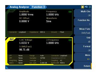
Figure 4-40 Analog Analyzer > Functions > SNR (Fast) menu page 1
