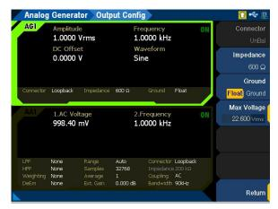
Figure 3-56 Analog Generator > Output Config menu page
