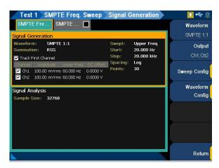
Figure 7-39 SMPTE Frequency Sweep > Signal Generation settings menu page
