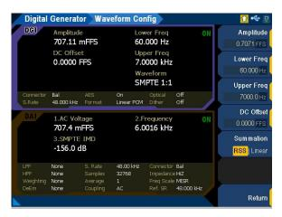
Figure 3-14 Digital Generator > Waveform Config menu page (SMPTE 1:1 waveform)
