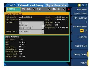
Figure 7-56 External Level Sweep > Signal Generation settings menu page
