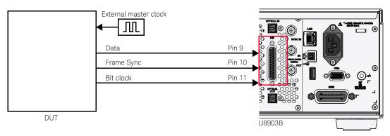
Figure A-5 DSI test configuration 2
