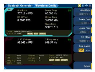
Figure 3-15 Bluetooth Generator > Waveform Config menu page (SMPTE 1:1 waveform)
