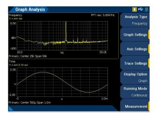
Figure 2-12 Graph analysis mode 2-panel view
