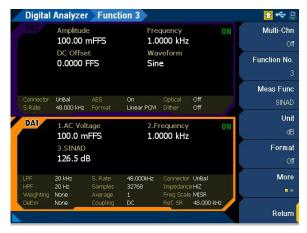
Figure 4-25 Digital Analyzer > Functions > SINAD menu page 1
