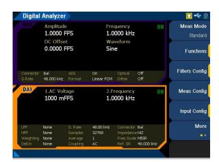
Figure A-10 Digital analyzer voltage measurement
