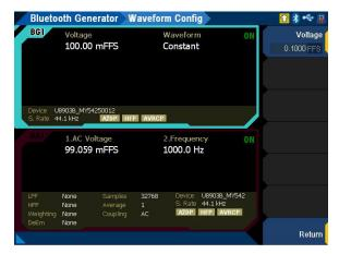
Figure 3-42 Bluetooth Generator > Waveform Config menu page (constant)
