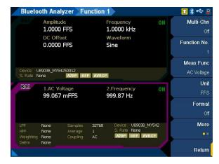
Figure 4-14 Bluetooth Analyzer > Functions > AC Voltage menu page 1
