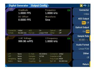
Figure 3-57 Digital Generator > Output Config menu page
