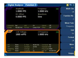
Figure 4-7 Digital Analyzer > Functions menu page 1
