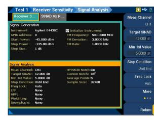
Figure 7-55 Receiver Sensitivity > Signal Analysis settings menu page
