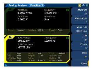
Figure 4-21 Analog Analyzer > Functions > THD+N Level menu page 1
