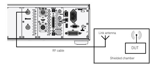
Figure 2-6 Wireless U8903B Bluetooth audio connection to DUT example
