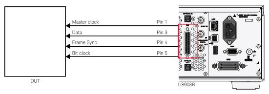
Figure A-4 DSI test configuration 1
