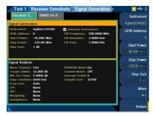
Figure 7-54 Receiver Sensitivity > Signal Generation settings menu page
