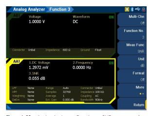
Figure 4-39 Analog Analyzer > Functions > SNR menu page 1
