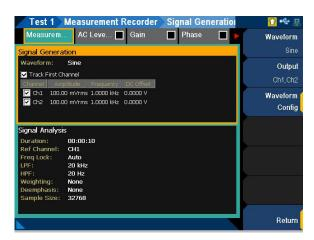
Figure 7-58 Measurement Recorder > Signal Generation settings menu page
