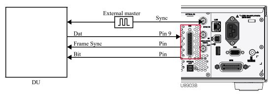
Figure A-6 DSI test configuration 3
