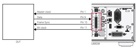
Figure A-8 DSI test configuration 5
