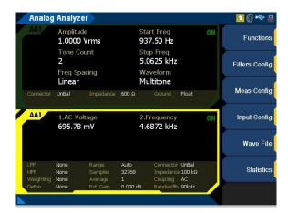
Figure A-12 Analog analyer multitone waveform measurement
