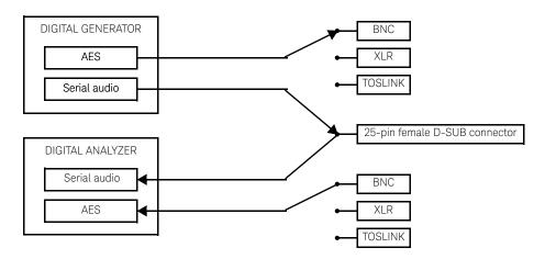
Figure 2-3 U8903B digital generator and analyzer block diagram
