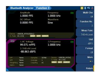
Figure 4-23 Bluetooth Analyzer > Functions > THD+N Level menu page 1
