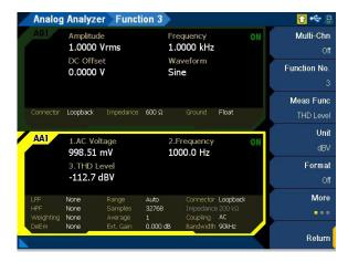
Figure 4-30 Analog Analyzer > Functions > THD level menu page 1
