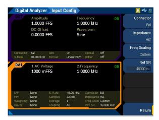
Figure 4-63 Digital Analyzer > Input Config menu page
