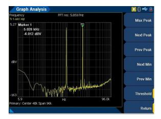
Figure A-13 Graph analysis for multitone spectrum
