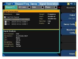
Figure 7-37 Stepped Frequency Sweep > Signal Generation settings menu page
