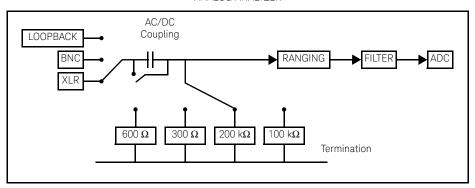
Figure 2-2 U8903B analog analyzer block diagram
