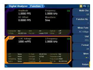
Figure 4-13 Digital Analyzer > Functions > AC Voltage menu page 1
