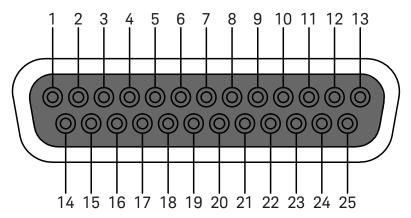
Figure A-2 25-pin female D-SUB connector
