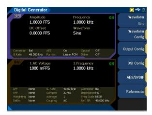
Figure A-9 Digital generator sine waveform generation
