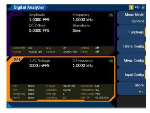
Figure 4-2 Digital Analyzer menu page (standard measurement mode)
