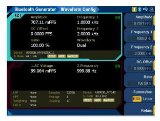
Figure 3-12 Bluetooth Generator > Waveform Config menu page (dual waveform)
