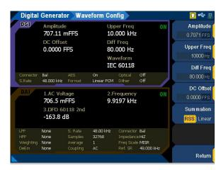
Figure 3-17 Digital Generator > Waveform Config menu page (IEC 60118 waveform)
