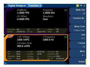
Figure 4-43 Digital Analyzer > Functions > Positive Peak menu page
