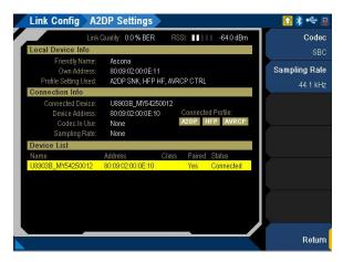
Figure 3-67 Bluetooth Analyzer > Link Config > A2DP Settings menu page
