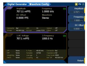
Figure 3-39 Digital Generator > Waveform Config menu page (stereo)
