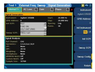
Figure 7-43 External Frequency Sweep > Signal Generation settings menu page
