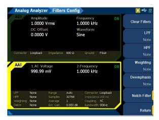
Figure 4-51 Analog Analyzer > Filter Config menu page
