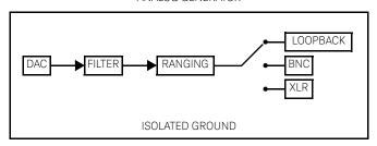
Figure 2-1 U8903B analog generator block diagram
