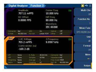
Figure 4-37 Digital Analyzer > Functions > DFD 60268 2nd menu page 1
