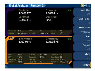
Figure 4-10 Digital Analyzer > Functions > Frequency menu page 1
