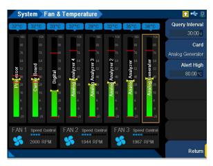
Figure 2-32 System > Fan & Temperature menu page
