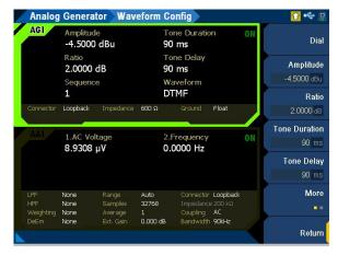
Figure 3-54 Analog Generator > Waveform Config menu page 1 (DTMF)
