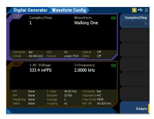
Figure 3-44 Digital Generator > Waveform Config menu page (walking one)
