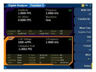
Figure 4-44 Digital Analyzer > Functions > Negative Peak menu page
