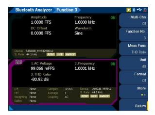
Figure 4-29 Bluetooth Analyzer > Functions > THD Ratio menu page 1
