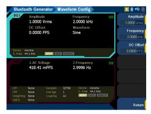
**Figure A-11** Bluetooth generator sine waveform generation
