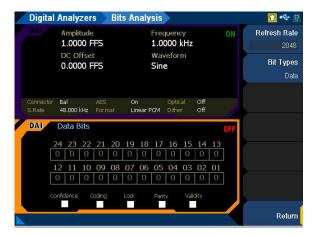
Figure 4-66 Digital Analyzer > Bits Analysis menu page 1
