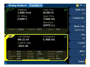
Figure 4-33 Analog Analyzer > Functions > SMPTE IMD menu page 1
