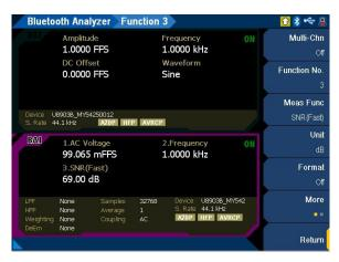
Figure 4-41 Bluetooth Analyzer > Functions > SNR (Fast) menu page 1
