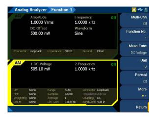
Figure 4-15 Analog Analyzer > Functions > DC Voltage menu page 1
