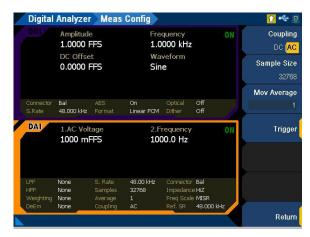
Figure 4-57 Digital Analyzer > Meas Config menu page
