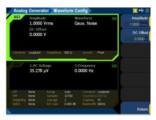
Figure 3-22 Analog Generator > Waveform Config menu page (Gaussian noise)
