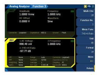
Figure 4-18 Analog Analyzer > Functions > THD+N Ratio menu page 1
