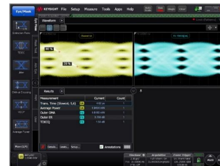
Figure 42. Optical 106.25 Gbaud PAM4 signal, generated using M8050A BERT and N7718C optical reference transmitter
