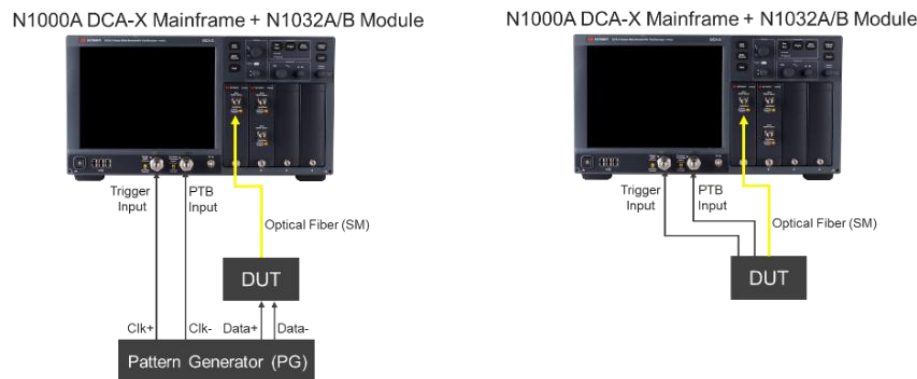
Figure 30. Typical setup for signaling rates > 112 Gbaud
