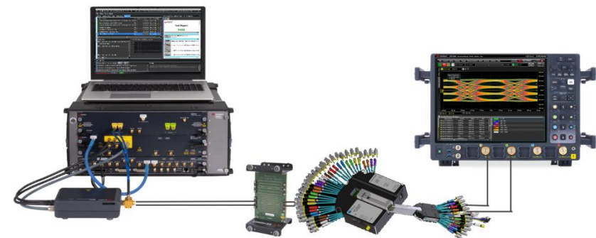
Figure 36. Setup configuration for C2M stressed eye calibration (host test)
