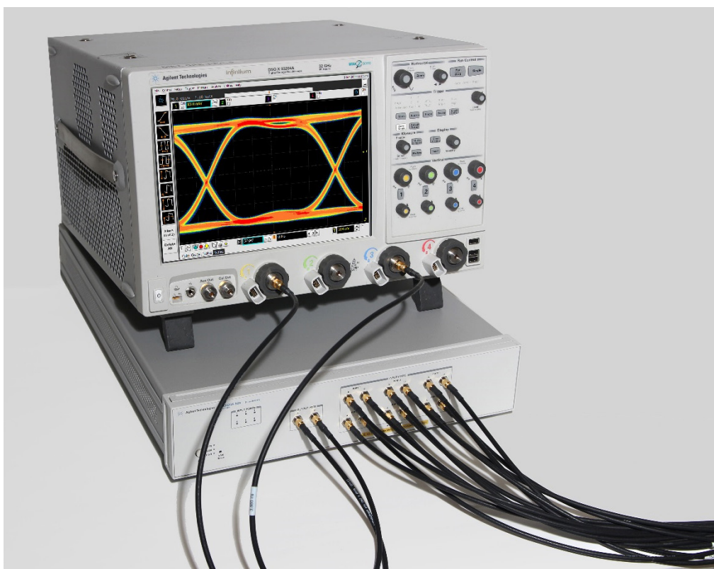
Figure 6. Automated testing for multi-lane digital bus interface through switching solution.
