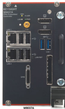
Figure 6 Front panel view of M9037A Embedded Controller
