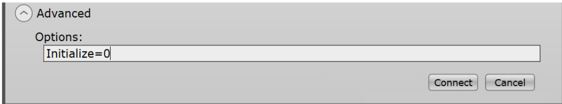
Figure 37 Setting option 'Initialize=0' to perform firmware update through SFP
