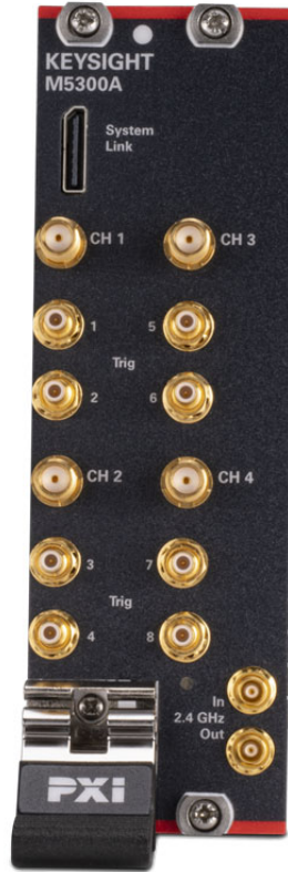
Figure 1 Front view of an M5300A High-Speed PXIe AWG module
