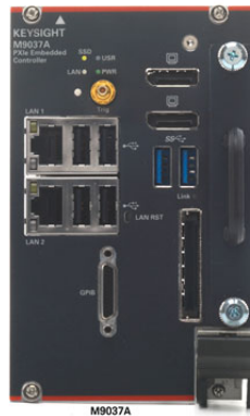
Figure 6 Front panel view of M9037A Embedded Controller
