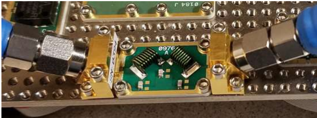
Figure 3. Lumped Element Filter with X-MWprobes
