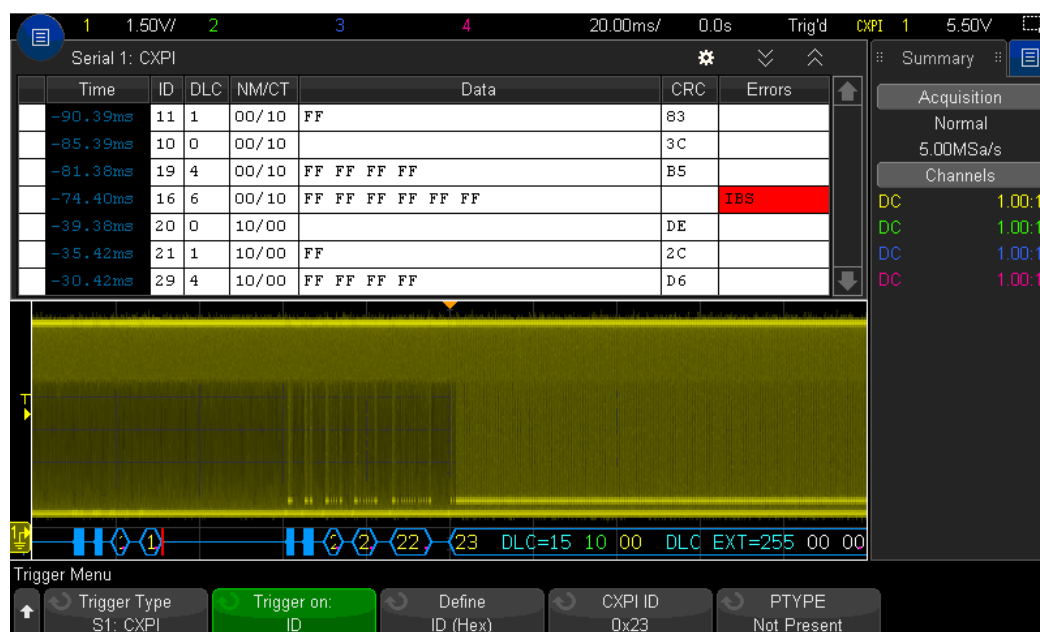
Figure 9. CXPI decode on an InfiniiVision X-Series oscilloscope.
