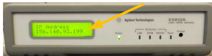
Figure 46 E5810B Front Panel showing IP Address
