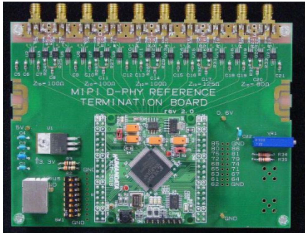
Figure 7 Sample MIPI D-PHY Reference Termination board (RTB)
