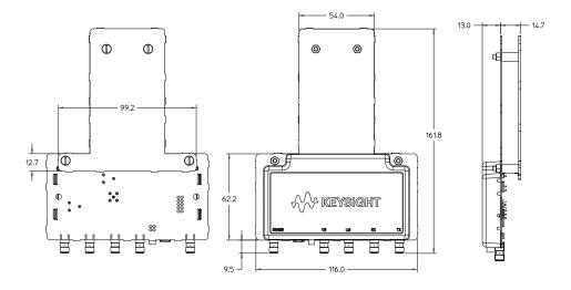
The N2135A 3-in-1 programmable NFC antenna provides 15 mm spacing between poller/listener coils.
