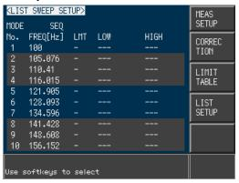
2. Set the trigger to manual mode by pressing Meas Setup hardkey, then cursor down to the TRIG field to select MAN
