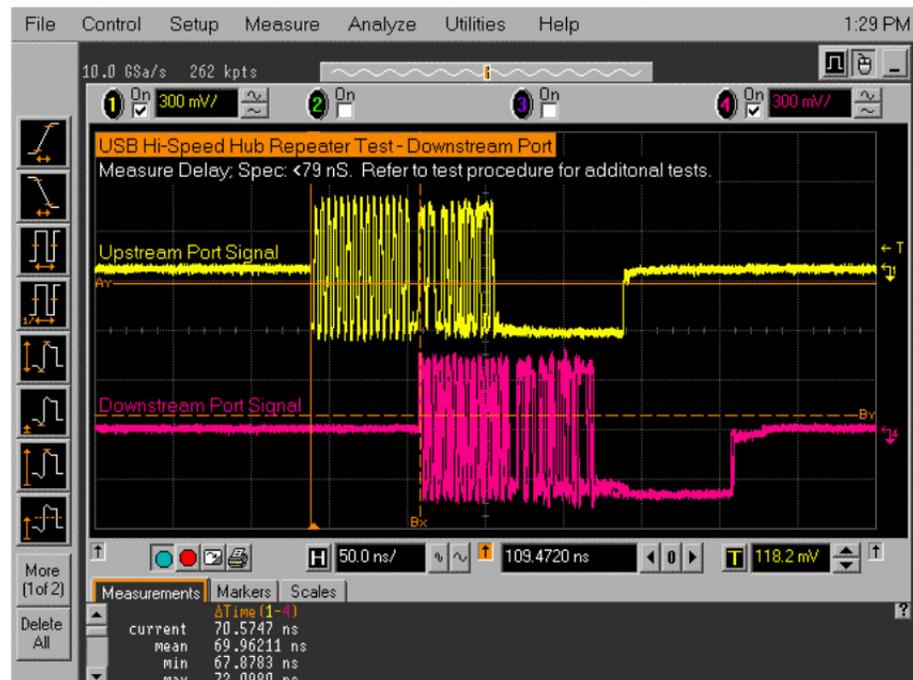
Measure the delay between the start of packet between the hub's upstream facing port (Channel 1) and the hub's down stream facing port under test (Channel 4) using the automatic measurement shown in .
