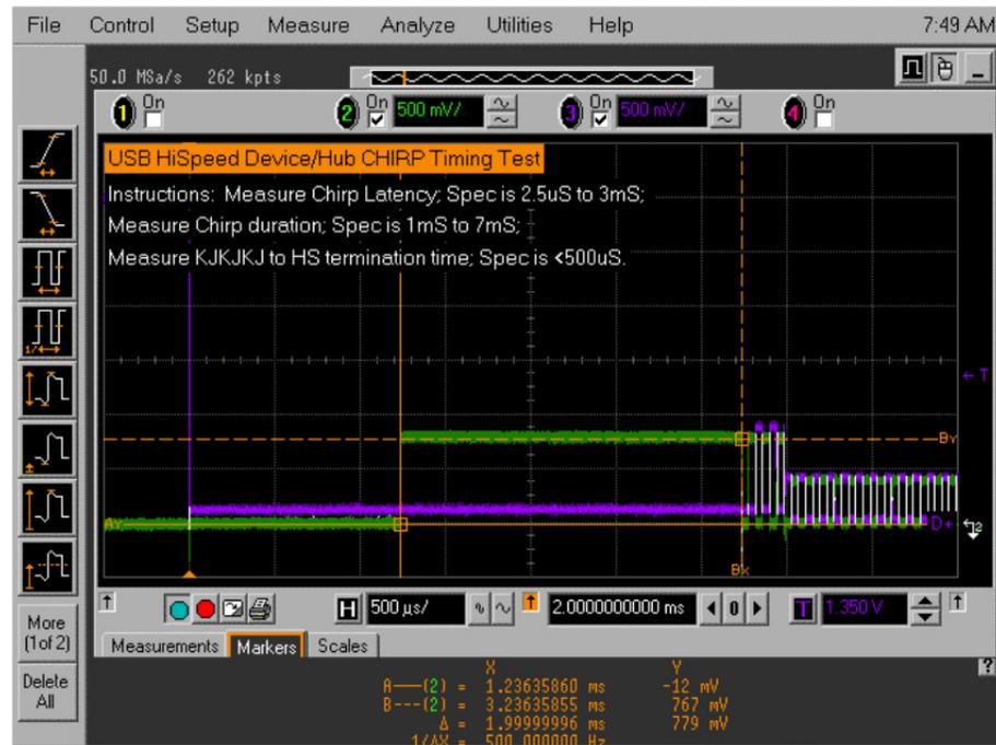
Using the markers, measure the time from the beginning of the last J in the CHIRP K-J-K-J-K-J (3 pairs of CHIRP-K-J's) to the time when the device turns on the Hi-Speed terminations, as shown in the following figure.
