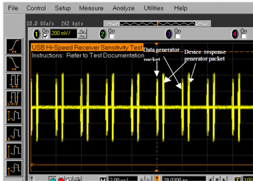
Reduce the amplitude of the data generator packets in 20 mV steps (on the generator before the attenuator) while monitoring the NAK response from the device on the oscilloscope.
