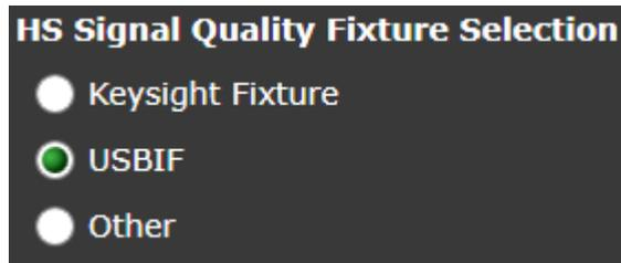
These settings affect ONLY the HS Signal Quality tests. They can be used to embed/de-embed the fixture. These settings DO NOT remove the differential probe or SMA cables.
