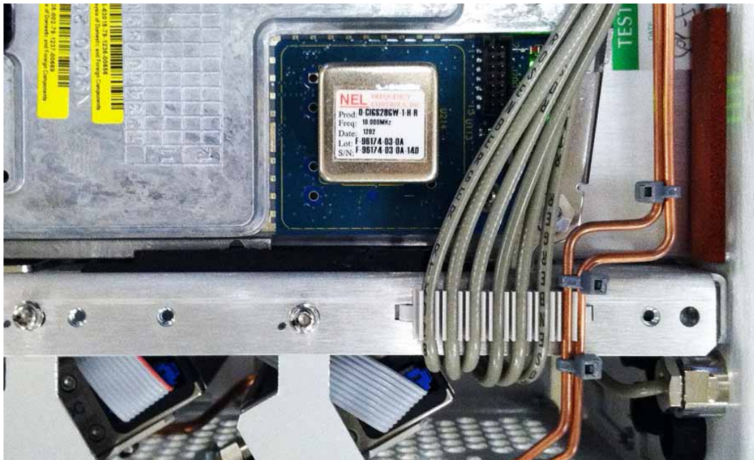
Figure 30 Dressing Cables to A16 Reference
