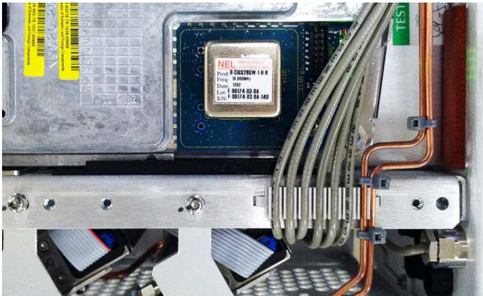
Figure 48 Dressing Cables to A16 Reference
