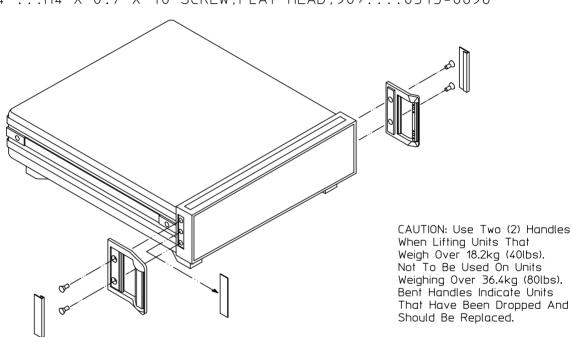
CAUTION: THIS KIT CONTAINS ONLY METRIC HARDWARE. INSTRUMENTS WITH METRIC CABINETS HAVE THE WORD "METRIC" CAST ON TOP OF THE FRONT FRAME (UNDER THE TRIM)."
