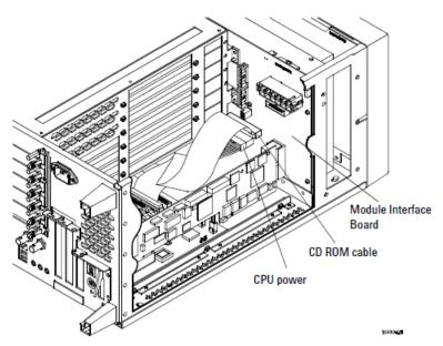
2 Remove 7 screws from the back of the CPU tray using a Torx T10 screwdriver.
