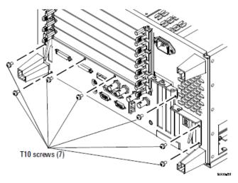
3 Use the tray levers to pry and disconnect the CPU board from the module interface board and slide the tray out being careful not to catch the loose cables on anything.
