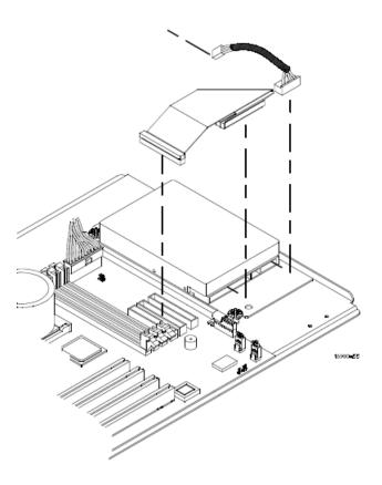
3 Using a Torx T15 screwdriver, remove the 4 screws that secure the hard drive to the hard drive plate. These screws are accessible through holes in the bottom of the CPU tray.
